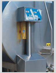
The circulation cleaning system was developed in the early 1990s. This fully-automated cleaning system (based on circulation cleaning) is mounted on the front side of the O-model.
